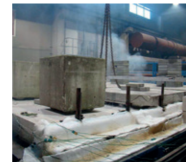
Op-Deck after 1 hour demonstrating no failure of insulation, integrity and load bearing capacity.
