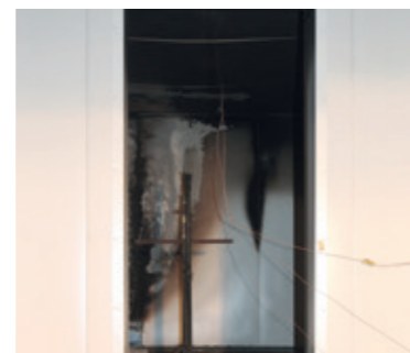
End of test showing limited internal damage and no evidence of flash-over conditions
