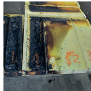
Panels at end of test with metal facings removed showing protective char formation on surface of insulation
