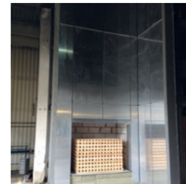
Test set up - Kingspan BENCHMARK façade panels with aluminium hook on cassette
