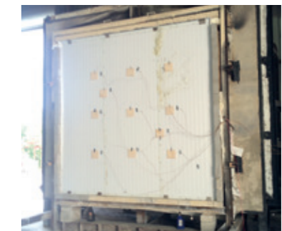
External face of QuadCore™ panel assembly after completion of 60 minute exposure.
