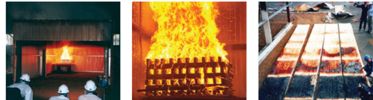
Test set up During test Inspection of protective char formation after test
