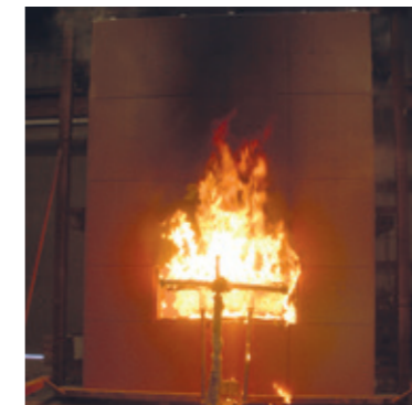
Fire exposure during test
