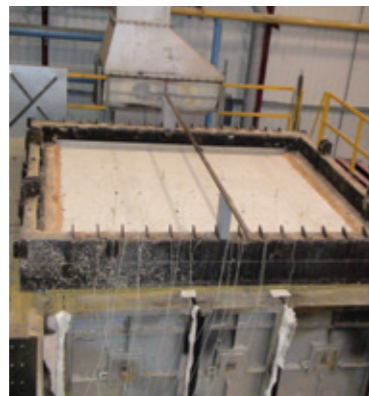
Ceilings / roofs (4m x 3m furnace)
