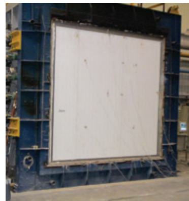
Vertical walls (3m x 3m furnace)
