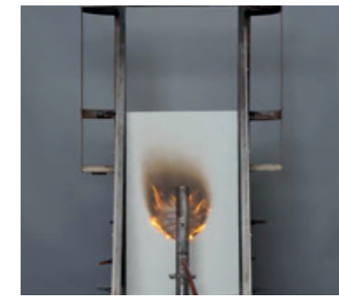
3 minute test in progress - note lack of surface burning and smoke emissions
