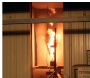
Test in progress - note burner adjacent to vertical panel joints
